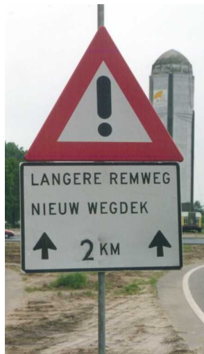
Figures 4b & 4c : Warning signs used in Derbyshire UK (Photo from Derbyshire Police) and on Dutch Motorways on Porous Asphalt - "longer braking distance, new road surface" to alert drivers of new road surfaces (Photo from DWW)
